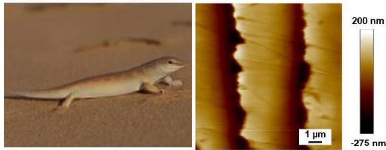
Figure 1: a) The sandfish ( Scincus scincus ) in its natural habitat. b) AFM scan of the scale of a sand-fish. The step like structures create anisotropic friction
