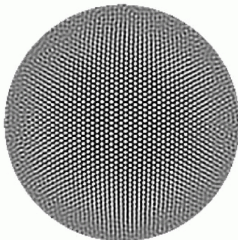
Figure 2. Hexagonal, self-organized convection cells (Bénard cells) in a heated fluid.
