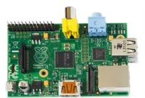
Scheme 1. Small low-power computer systems can play a key role in the Internet of Chemical Things. The Arduino (left) is used for inexpensive sensor and robotics applications. More powerful systems such as Raspberry Pi (right) are better suited for data processing and calculations.
