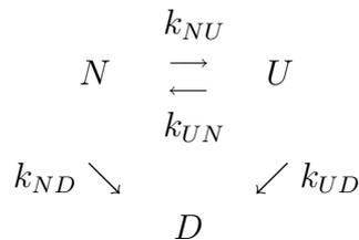
where  $k_{NU}$ ,  $k_{UN}$ ,  $k_{UD}$ ,  $k_{ND}$  denote rates of the corresponding reactions. Additionally a substrate S is involved, which is contained in the inflow and is degraded depending on the concentration of native enzymes.
